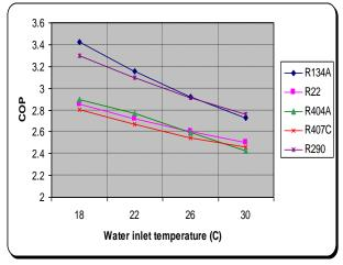
Figure 6: Variation of first law efficiency in terms of coefficient of performance (COP) vs. condensing water inlet temperature of different refrigerants
