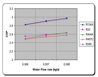
Figure 5: Variation of first law efficiency in terms of coefficient of performance (COP) vs. condensing water flow rate of different refrigerants
